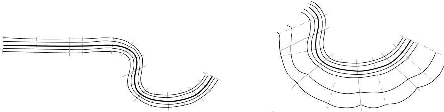
Fig. 7 Continuous approximation of the distance function obtained by using Algorithm 2 with factors of degree n = 1 (left), enlarged (right)
