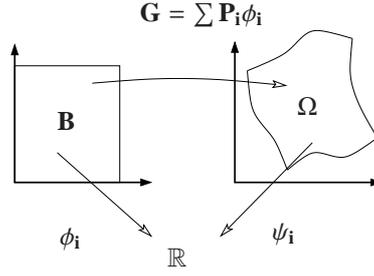
Figure 1: Two-dimensional parameterization  $\mathbf{G}$  with parameter domain  $\mathbf{B}$ , physical domain  $\Omega$  and basis functions  $\phi_i$  and  $\psi_i$
